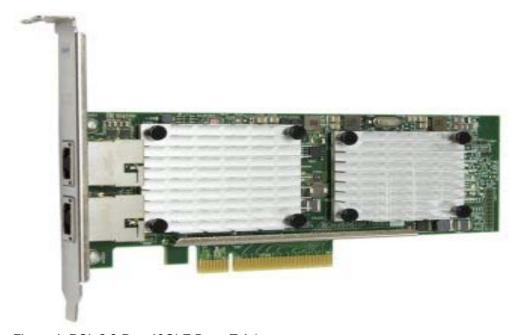
Figure 1. PCle2 2-Port 10GbE Base-T Adapter
